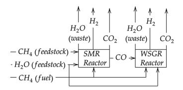
Figure 3. Steam reforming process
