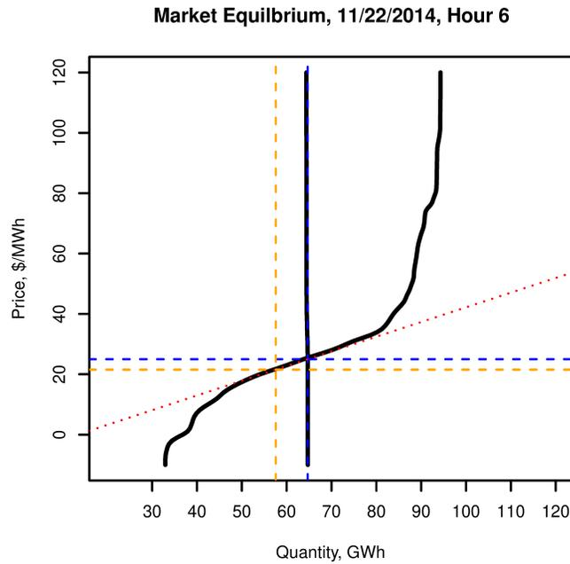
Figure 5: The reconstructed market supply and demand curves, in black, for a sample hour form the equilibrium price. The equilibrium is denoted by the dashed blue lines. The calculated merit order effect for a one unit increase is shown by the dashed red line. Walking down the merit order effect from the equilibrium shows the expected price reduction at with the yellow dashed lines.
