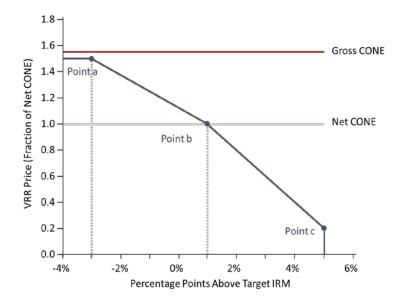
Figure 3. Status Quo VRR curve; 1) Point a is where 1.5 X Net CONE = Target reserve margin - 3%; 2) Point b is where Net CONE = Target reserve margin + 1%; 3) Point c is where 0.2 X Net CONE = Target reserve margin + 5%
